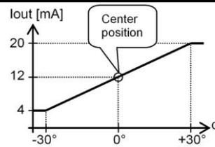
Default 0°: horizontal (label upwards), no acceleration applied.
