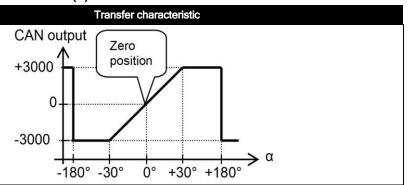
Default 0°: horizontal (label upwards), no acceleration applied. To eliminate mounting offsets the sensor can be zero-ed within ±5° tilt (by the CAN object dictionary)
