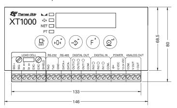
All dimensions in mm. Connection terminals shown are for version XT1000-SO-AN.
