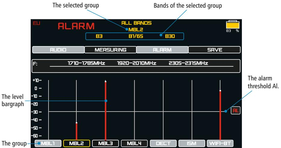
The groups will be displayed at the bottom of the screen. The signal levels by groups are displayed on the bargraphs. By pressing the joystick to the left and right, the user can choose a group and see which bands belong to it.
