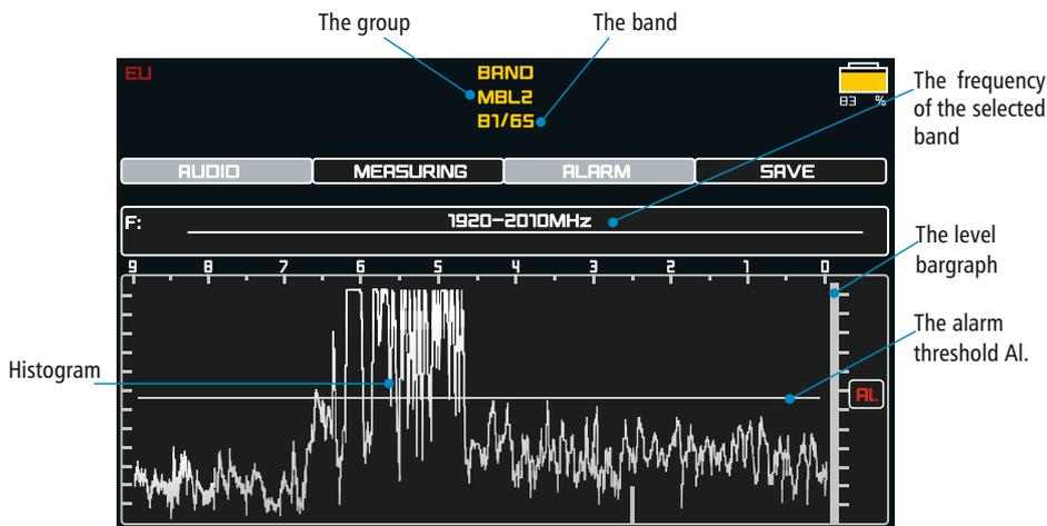
In addition to the level bargraph, a **histogram** is displayed in this mode. The histogram is a graph where the history of the signal level for a certain time period is shown. It allows you to not miss the signal when you approach, or move away from the transmitter, or when it has a non-continuous mode of operation.
