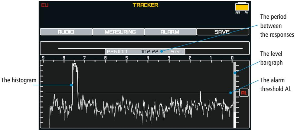
The **alarm threshold** can be adjusted, and the **ALARM** and **AUDIO** functions can be switched on. A subsequent **pressing of the joystick button** selects the ALL BANDS mode.
