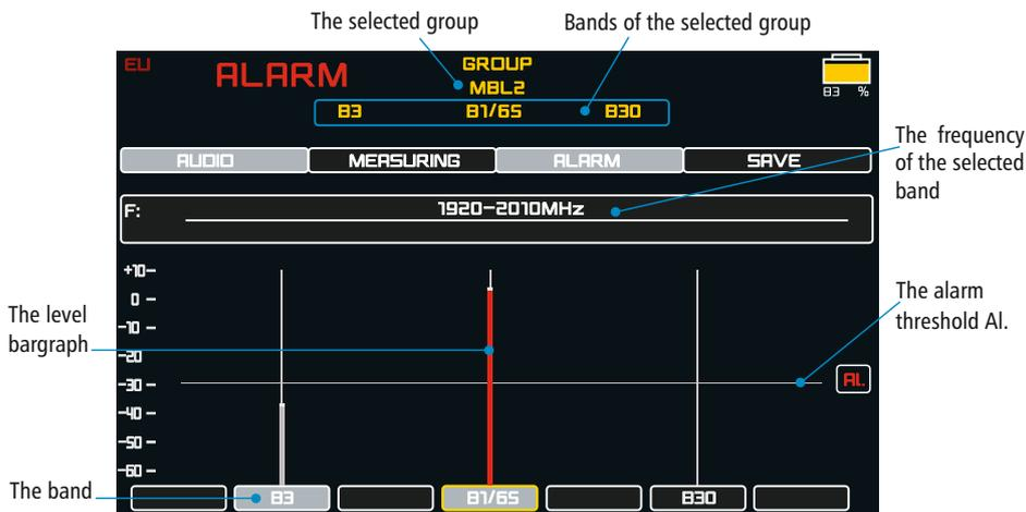
The **alarm threshold** can be adjusted, and the **ALARM** and **AUDIO** functions can be switched on. A subsequent **pressing of the joystick button** selects the **BAND** mode where a band can be inspected
