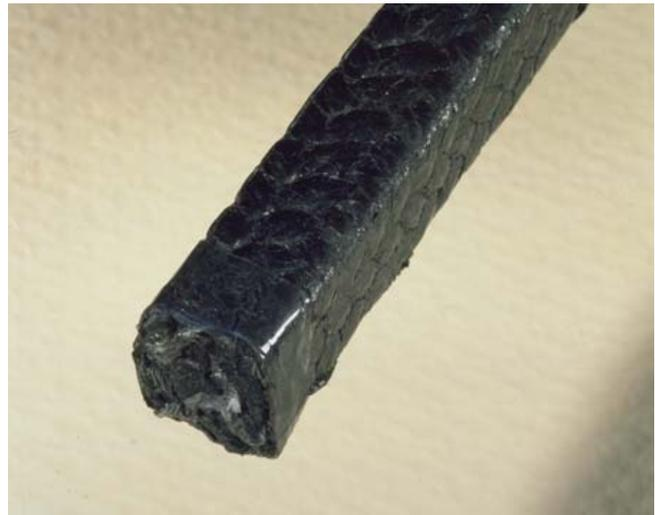
A combination of selected glass fibre yarns with graphite lubricant impregnation, Klingerlock braided to produce an efficient alternative to asbestos in valve applications and static sealing duties eg. caulking purposes.
