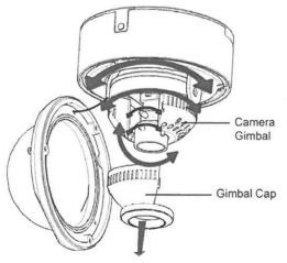
Open the bubble cap and move the camera gimbal to left, right and up, down to set the viewing direction. After set the viewing direction, open the gimbal cap like the arrow diection and adjust the viewing angle.
