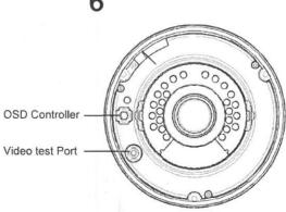
Set the desired OSD feature by using the OSD controller. (Refer the SOD manual to set up the desired OSD) in case of a installer has portable monitor, connect the video jack to the video test port to set up the OSD.
