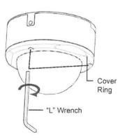
Tighten the screw by using the "L"wrench and complete the installation.
