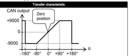
Default 0°: horizontal (label upwards), no acceleration applied. To eliminate mounting offsets the sensor can be zero-ed within ±5° tilt (by the CAN object dictionary)
