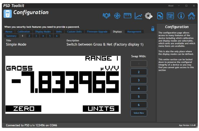
Configure the available Display Mode slots with the required Display Modes.
