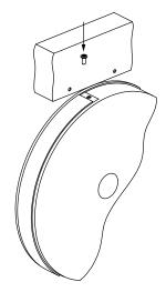
③ Use the included fastener (ARC00) and fasten down the right side of the scale. Use the recommended torque from the **Table of recommended fastener tightening torques.**
