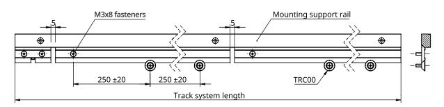
Recommended use of M3x 8 (CBSM3-8 Misumi). For more information see **<u>Table of recommended fastener tightening</u>** torques at <u>**RLS Media center.**</u>
