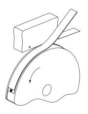
(2) Apply the scale alongside the installation lip while slowly rotating the shaft and peeling off the liner.
