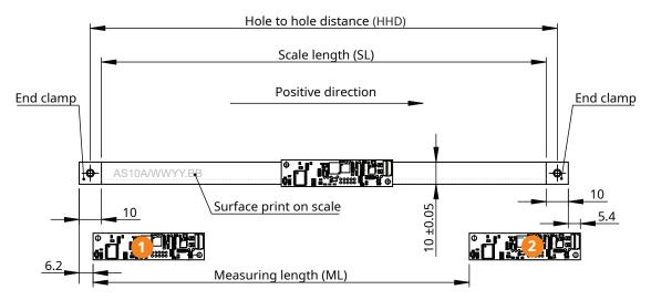
ML = SL – 38 mm HHD = SL + (6 mm ±1 mm) SL tolerance = ±(0.5 mm +0.04 mm/m) \* Scale surface print does not represent the actual ordering code. For orientation purpose only.
