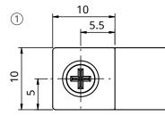
Prepare the mounting surface. Drill the holes to the mounting surface as shown above.
