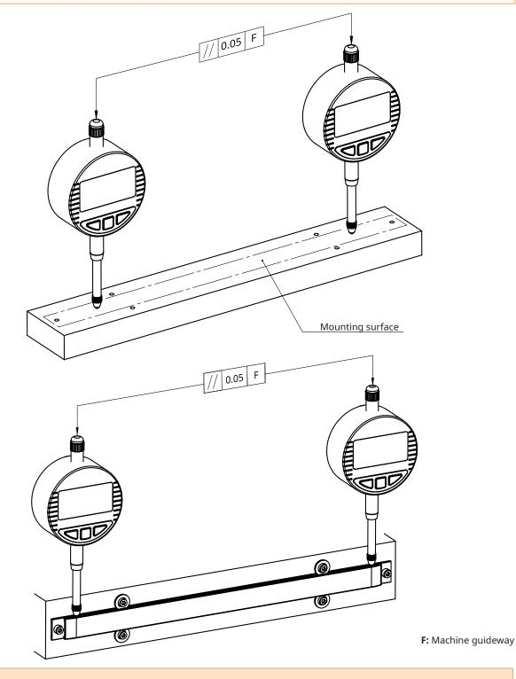
To achieve specified performance, maintain the mounting surface and the readhead guideway inside 0.05 mm parallelism according to the machine guideway.
