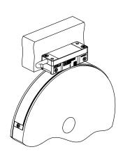
(5) Align the readhead according to the tolerance specification (radial, axial, tangential offsets). A simple 0.3 mm thick plastic shim can be used to set up the air gap between the scale and the readhead.
