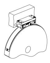
(6) Align the readhead according to the tolerance specification (radial, axial, tangential offsets). A simple 0.3 mm thick plastic shim can be used to set up the air gap between the scale and the readhead.
