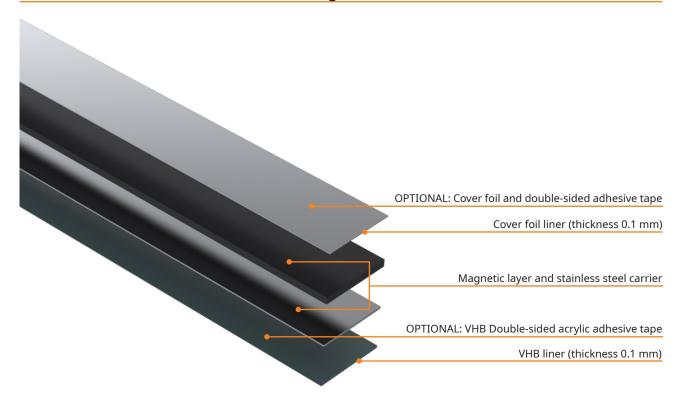
Structure of SAS10 absolute magnetic scale on a solid substrate
