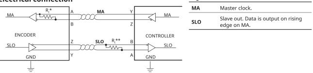
\* The MA and SLO lines are 5 V RS422 compatible differential pairs. The termination resistor on the MA line is integrated inside the encoder.
