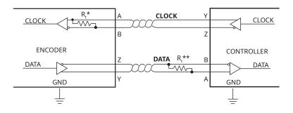
\* The CLOCK and DATA lines are 5 V RS422 compatible differential pairs. The termination resistor on the CLOCK line is integrated in the encoder.
