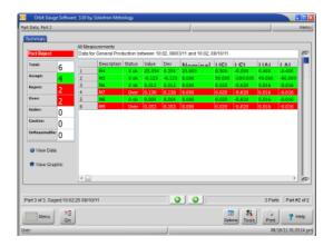
All parts data is stored within the SI9500 and can be inspected inside the software. Text export is available for integration into SPC packages.
