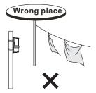
Remove all obstructions ( trees, clothes lines, etc.) between Transmitter and Receiver.
