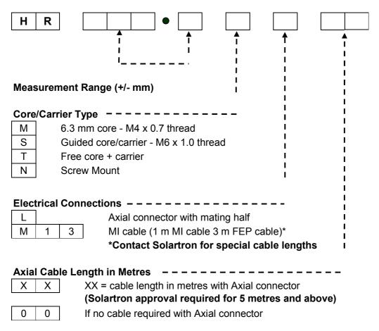
Contact Solartron for cable options with BICM
